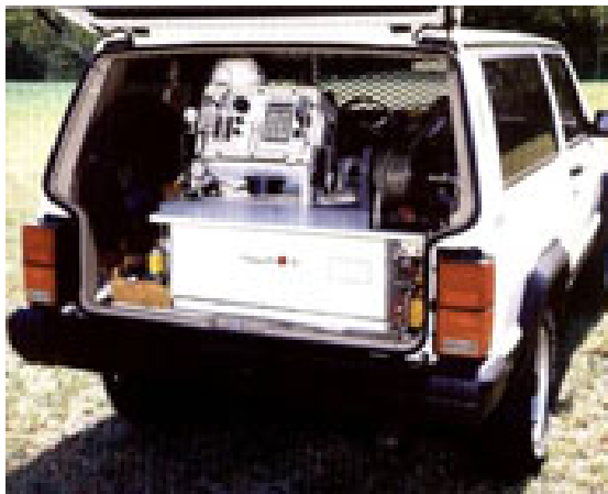
Fig. 3A-Chandler Eng. Gas Chromatograph in Jeep
