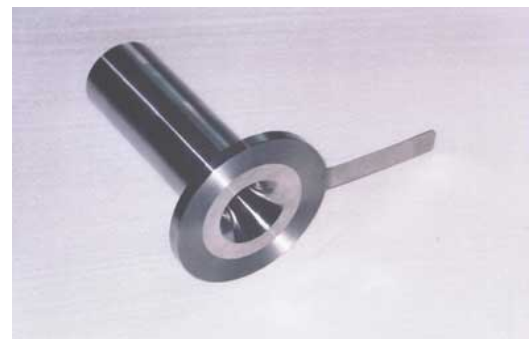
Figure 3. Toroidal Throat Nozzle Construction and Installation Specifications from ASME/ANSI MFC-7M [11]
