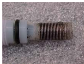
P 2 O 5 contaminated With Glycol
