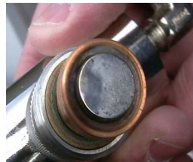
Mirror outside of Instrument coated With Glycol
