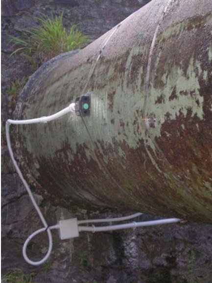
Figure 7. Single Path Clamp-On System on a Large Pipe.
