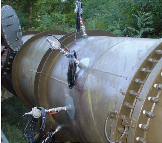
Figure 10. A Multipath Insertion Type Transducer System.
