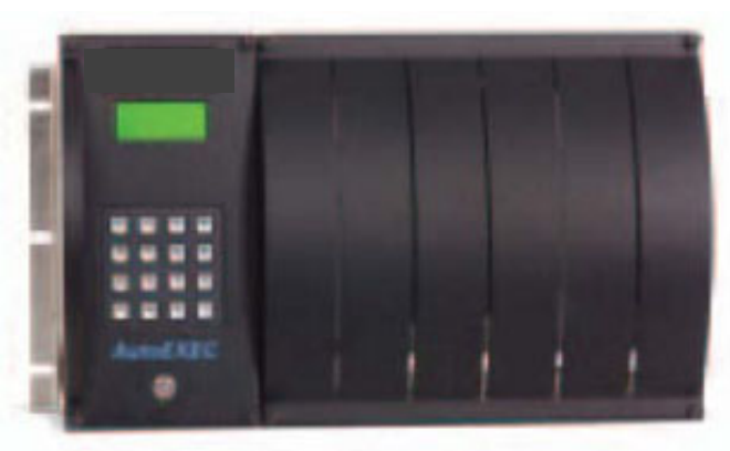
Figure 4.0 Typical PLC Based Flow Computing System
