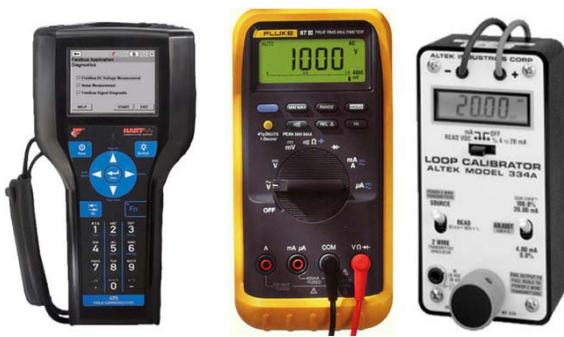
Figure 16. HART Communicator, Digital Multimeter, mA Loop Simulator
