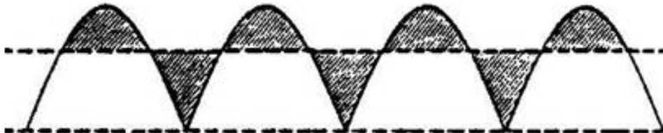
Figure 12. Limiting high amplitude and eliminating low amplitude can convert a sine wave to a square wave.
